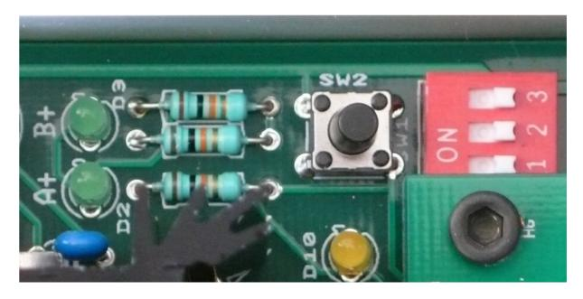
All switches SW1 "off": minute impulse, slave max. 12.00h indication, impulse time 0,6 sec.
