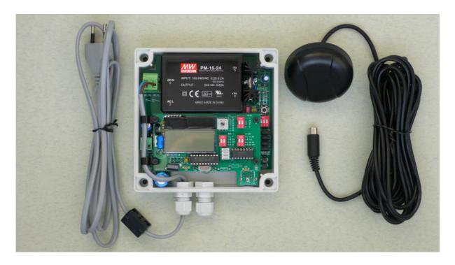
The SR500 can be used on places where alternating current is available. The small GPS receiver is equipped with five meter cable.
